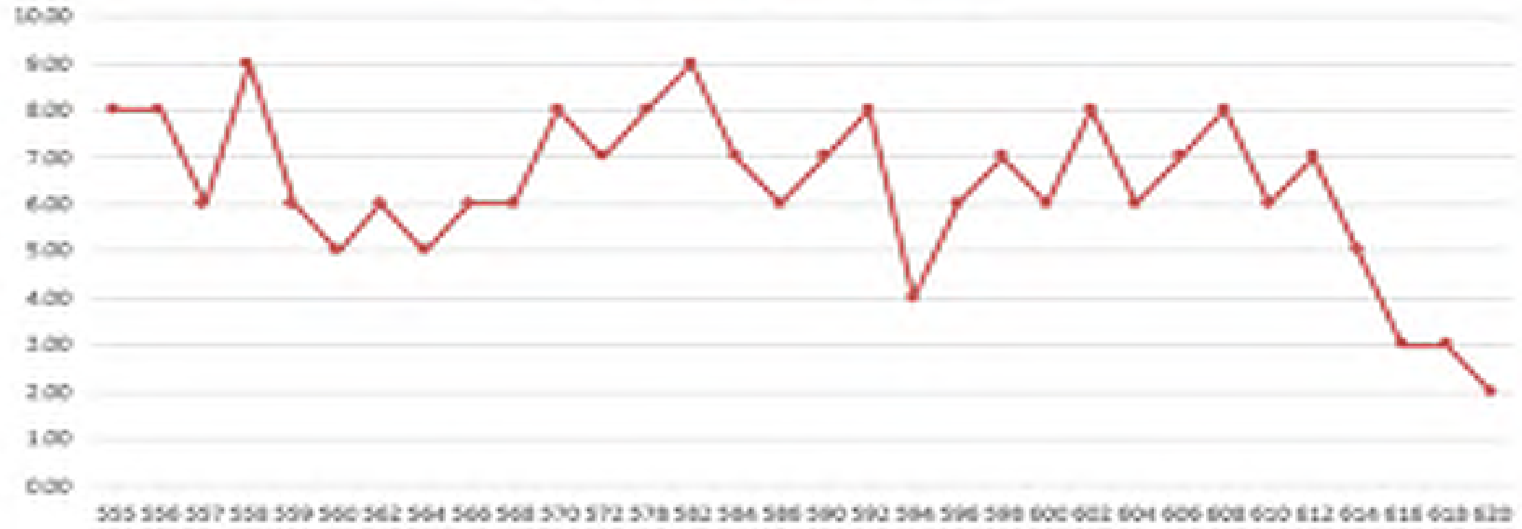
Vertical Displacement of Built Tunnel
